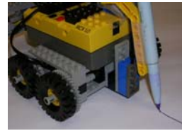
Figure 2: Penbot with pen in drawing position
